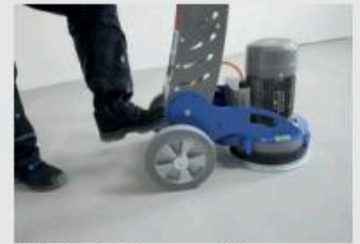
With footrest for easy tilting of the machine
