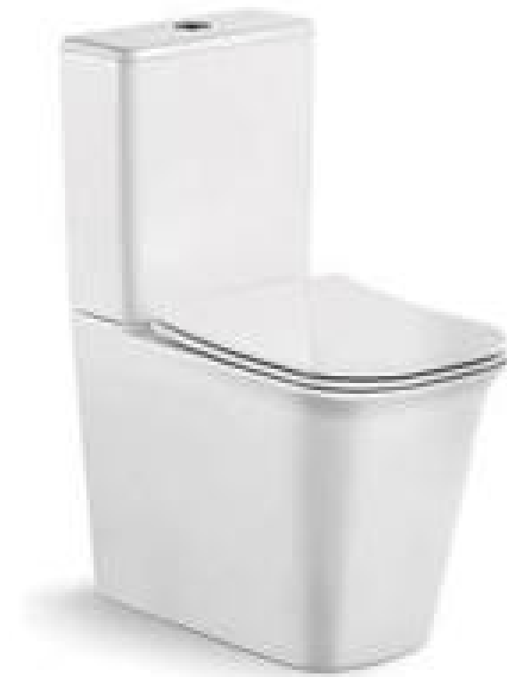
31022972 Washdown two-piece toilet Full back to wall Size: 620x345x800mm S-trap: 250mm Roughing-in P-trap: 180mm Roughing-in
