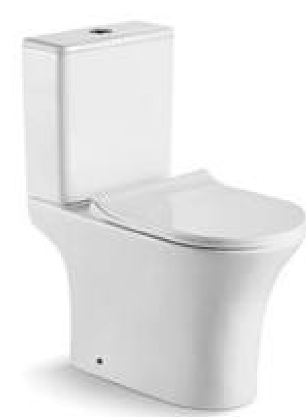
3096-2970 Washdown two-piece toilet Size: 650x340x770mm S-trap: 250mm Roughing-in P-trap: 180mm Roughing-in
