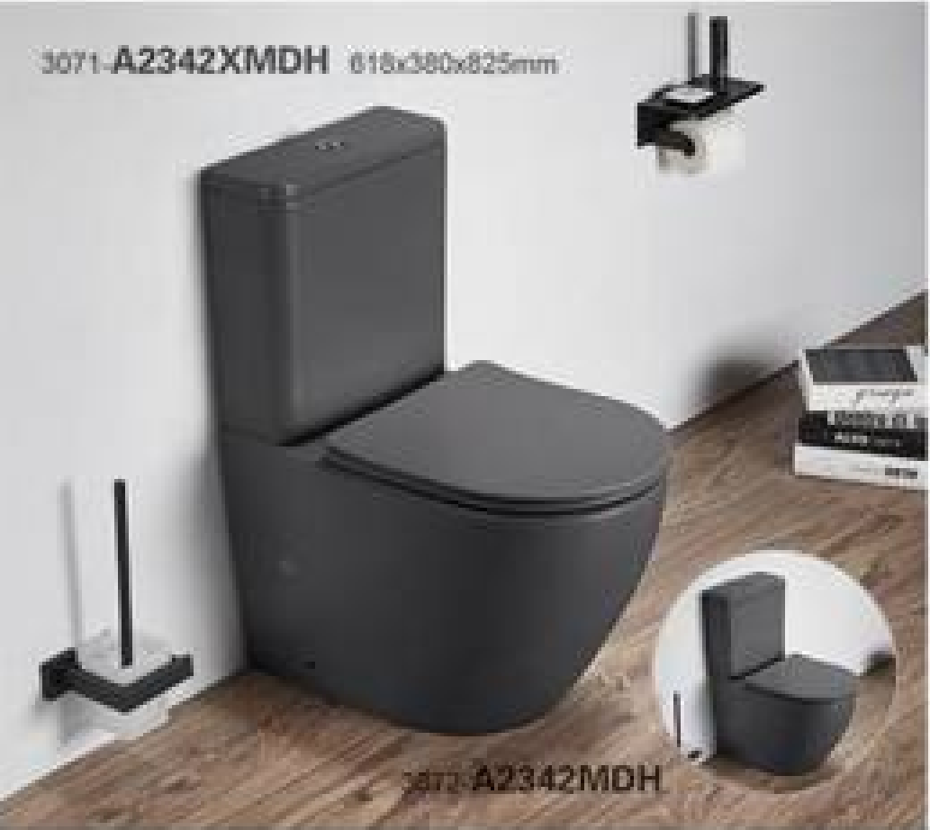
A 2342 Washdown two piece toilet. Size: 618x380x825mm S-trap 250mm Roughing-in P-trap 180mm Roughing-in
