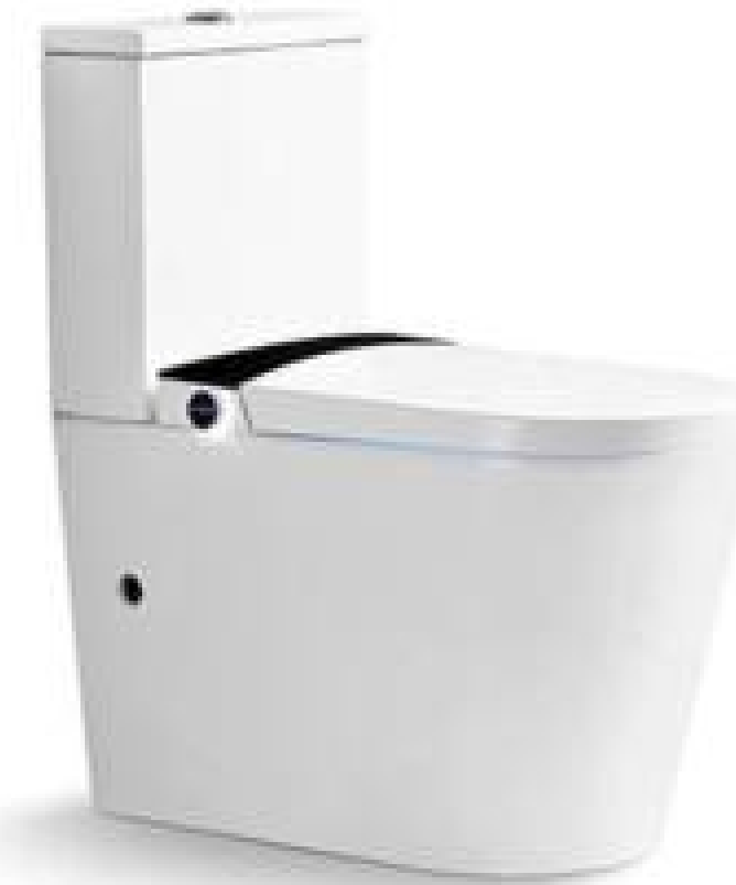
3201-T5-P Intelligent toilet Size: 730x370x840mm P-trap: 180mm Roughing-in
