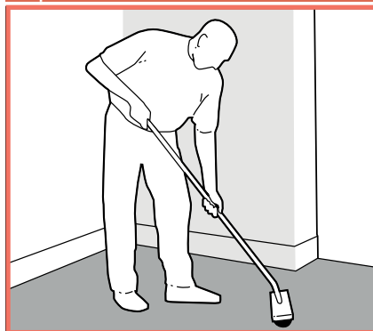
3 COMPRESS CARPET TO UNDERLAY
