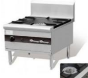
Stock Pot Stove Model GRP-SP-1 Dimensions(mm) 600*160*500-200 Burner Rating(kW) 24 N.W.(kg) 67 Gas Source LPG 2800Pa NG 2000Pa
