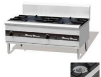
Stock Pot Stove Model GRP-SP-2 Dimensions(mm) 1200*160*500-200 Burner Rating(kW) 24*2 N.W.(kg) 138 Gas Source LPG 2800Pa NG 2000Pa
