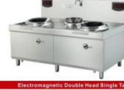
Electromagnetic Double Head Single Tail Fried Stove Model GR-XDL400-1 GR-XDL400-1A GR-XDL500-1 Dimensions(mm) 1500*900*(800+400) 1600*1100*(800+400) 2000*1100*(800+400) Volt. 380V 380V 380V Power(kW) 12*2/15*2 12*2/15*2 15*2/18*2 Wok Size(mm) Built-in \pm 500mm wok Built-in \pm 500mm wok Built-in \pm 600mm wok
