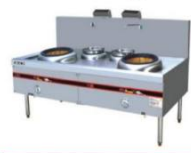
Chinese Cooking Range (2 Burners 2 Warmers) Model GR-BG-2022 Dimensions(mm) 2000*1000*1150 Volt./Power 220V 50Hz/550W N.W.(kg) 320 Wok Size(mm) Built-in \pm 500mm wok
